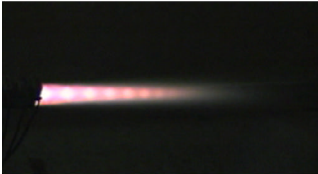
PLATE 1: Supersonic Flame during Pilot Hydrogen injection
