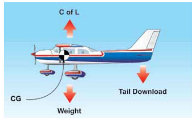
Figure 2-21. Downward Force on the Tailplane.
