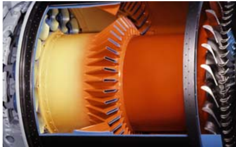
Above | View inside a BMW 003 unit. Visible from left to right: combustion chamber with air blending fins, cooling stators and turbine, 1978.
