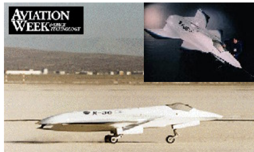
Figure 28 - X-36 Tailless, Thrust-Vectoring Drone Research Aircraft
