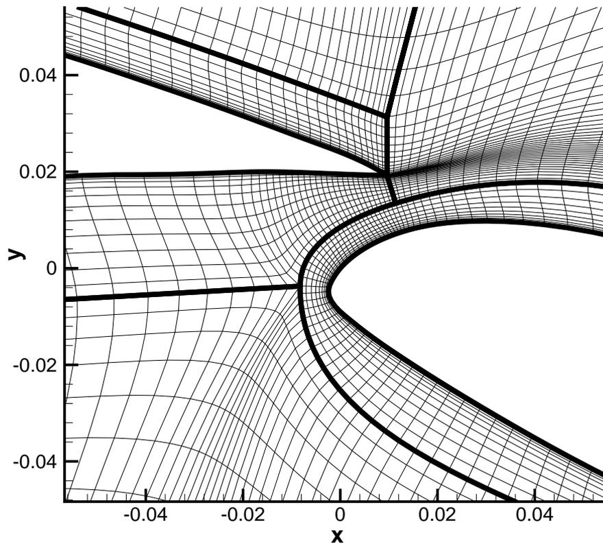
Figure 1: Computational grid and block boundaries in vicinity of flap nose
