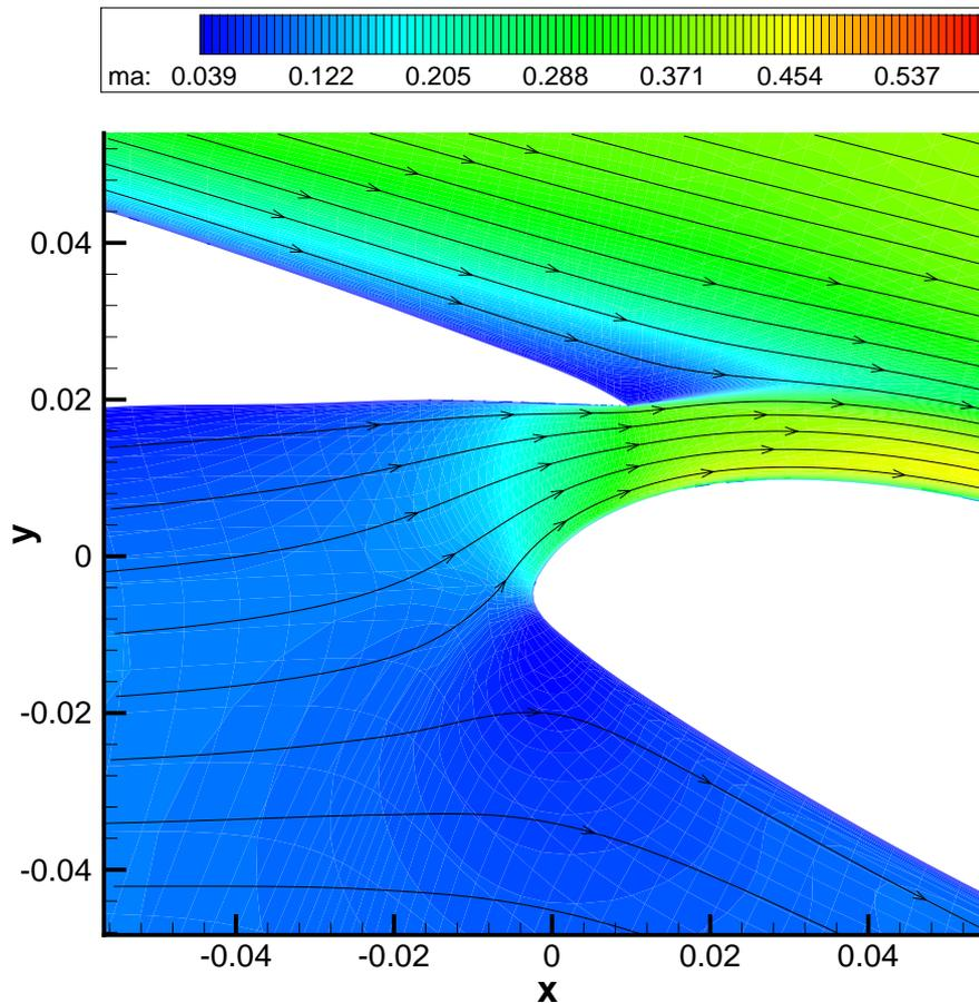
Figure 2: mach number and streamtraces in vicinity of flap nose
